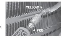
(C) Barely thread the middle manifold (charging/yellow) hose to the male fitting of AC Leak Freeze PRO injector. Do not thread to the point of depressing the Schrader core. (D) For best results raise the AC Leak Freeze PRO canister above the service port. (E) Briefly crack open manifold high side valve to purge air out of hoses, close manifold high side valve; while quickly tightening the charging hose fitting to the inlet fitting on the injector.
