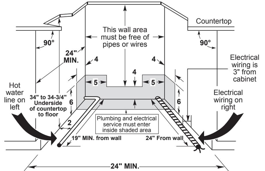
**NOTE:** Dishwasher must not be installed more than 10 feet from sink for proper drainage. All plumbing and electrical work must be in accordance with local codes. Dishwasher includes drain hose and leveling legs.
