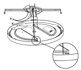
Twist and lock fixture into the mounting bracket in the Lock direction of the arrows next to the dots.
