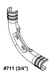
The PEXRITE® #710 & #711 snap onto 1/2" and 3/4" CTS tubing, respectively, to provide support for a 90° change of direction, and can be attached directly to joists, framing, etc. Compatible with all PEX tubing manufacturers.
