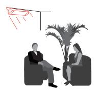
Install fixture to heat the area from the "cold side" if possible. This helps compensate for increased body heat losses due to exposure. Warm floors reradiate heat. Warmer air rises from floor. Some heat reflects from floor. Mounting a heater directly over a table or other obstruction will block the energy, primarily heating the object. It is best to move heater to the side, allowing complete body and floor coverage.
