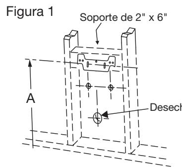
2. Hold the steel hanger, supplied, against the wall and centered over the waste outlet hole at suggested height (29-3/8"-30-5/8") and mark location with a pencil. Mount bracket on the wall by inserting lag screws through the 4 upper holes of the bracket as shown in (Fig. 2).
