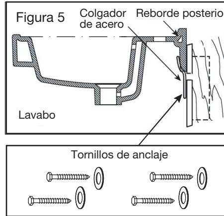
5. Lag bolts with washers sized to fit shall be installed in lavatory anchor holes located on the back sides of the sink. The anchor bolts must be installed and tightened snugly to prevent the lavatory from lifting off the wall, (Fig. 6). A pilot hole may need to be drilled to securely anchor the lag bolts. Make sure the lavatory is leveled before tightening these bolts.
