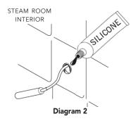
**PARNING** Insure a minimum of 1/4" of the temperature probe is exposed to the air. Failure to do so may interfere with the ability to sense tempera-ture and may result in excessive steam room temperatures.
