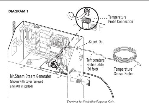
5. Route the end of the probe cable with the temperature probe through the wall into the steam room as shown in Diagram 2.
