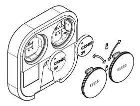
Replace the battery door and lock in place.
