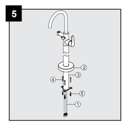
Place the assembly with the flexible supply lines (1) through the prepared hole. Then holding the escutcheon (2), secure the standpipe (3). Note: If mounting into wooden floor, secure the standpipe (3) using screws (4) only (wall plugs are not needed). If mounting into solid floor, mark the position of holes first and then secure the standpipe (3) using anchors (5) and screws (4). Where requried ensure correct anchors for your floor type are used.
