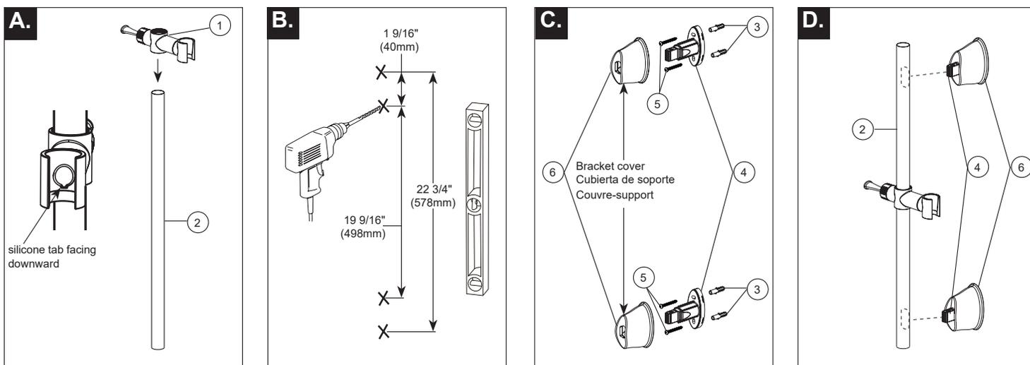
**A.** With the Slide Mount's (1) silicone tab facing downward, slide the Slide Mount (1) onto the wall bar (2).
