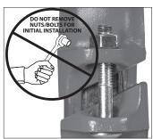
1. DO NOT DISASSEMBLE THE COUPLING: Style 009N FireLock EZ™ Installation-Ready™ Rigid Couplings are designed so that the installer does not need to remove the nuts and bolts for initial installation. This facilitates installation by allowing the installer to directly insert the grooved end of mating components into the coupling.
