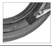
**3a.** If any conditions listed in the "NOTICE" on the following page are met, apply a thin coat of a compatible lubricant only to the gasket sealing lips. Refer to the "Lubricant Compatibility for Gaskets" table below.
