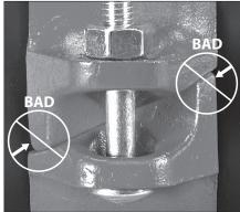
IMPROPERLY ASSEMBLED JOINT
