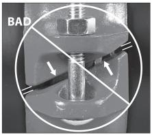
IMPROPERLY ASSEMBLED JOINT
