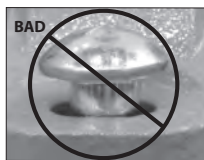
OVAL NECK OF BOLT NOT SEATED PROPERLY
