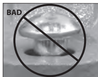
OVAL NECK OF BOLT NOT SEATED PROPERLY
