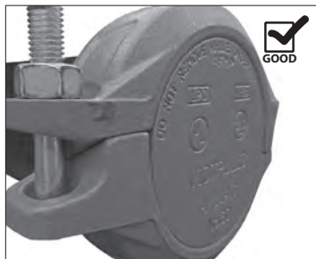
GOOD ASSEMBLY (END CAP IS SEATED WITHIN THE COUPLING WITH THE CORRECT SIDE FACING OUT AND COUPLING BOLT PADS ARE IN METAL-TO-METAL CONTACT)
