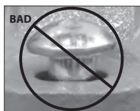
OVAL NECK OF BOLT NOT SEATED PROPERLY
