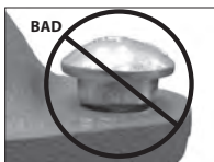
OVAL NECK OF BOLT NOT SEATED PROPERLY
