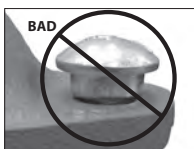
OVAL NECK OF BOLT NOT SEATED PROPERLY
