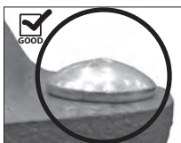
OVAL NECK OF BOLT SEATED PROPERLY
