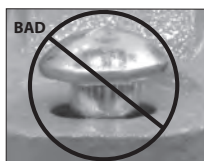
OVAL NECK OF BOLT NOT SEATED PROPERLY
