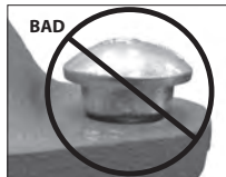
OVAL NECK OF BOLT NOT SEATED PROPERLY
