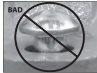
OVAL NECK OF BOLT NOT SEATED PROPERLY
