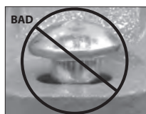
OVAL NECK OF BOLT NOT SEATED PROPERLY
