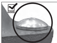
OVAL NECK OF BOLT SEATED PROPERLY
