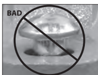
OVAL NECK OF BOLT NOT SEATED PROPERLY
