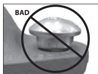
OVAL NECK OF BOLT NOT SEATED PROPERLY
