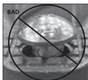
OVAL NECK OF BOLT NOT SEATED PROPERLY
