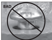
OVAL NECK OF BOLT NOT SEATED PROPERLY
