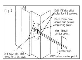
Mortise 7/32" deep or until the strike box, reinforcing strike and strike plate fits inside mortise and flushwith the door frame. (fig. 5)
