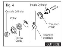
into the deadbolt. Align slot of inside cylinder with notch in threaded collar. Keeping tailpiece vertical and curved toward the right side of hole, insert inside cylinder with threaded collar into the deadbolt. Attach cylinders using two #10-32 x 2-1/4" flat head machine screws. Tighten screws. Do not insert key during this procedure. (fig.4)
