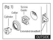
b. Place turnpiece mounting plate on inside of door as shown. The side with "TOP" marked on plate should be against the door. Attach cylinder using two #10-32 x 1-7/8" pan head machine screws. Insert screws through mounting plate, deadbolt, screw guide and collar into the cylinder. Tighten all screws. (fig. 2)
