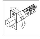
plate/bolthead assembly 180° until it stops. Unit is now ready for installation in a 2-3/4" backset configuration.
