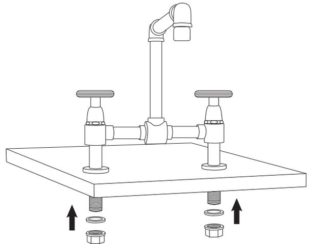
4. Connect the main water supply lines to the faucet. Apply plumber's tape or thread sealant to the threads before tightening. Use an adjustable wrench to tighten, but be careful not to overtighten. Ensure that you are connecting the hot and cold lines appropriately.
