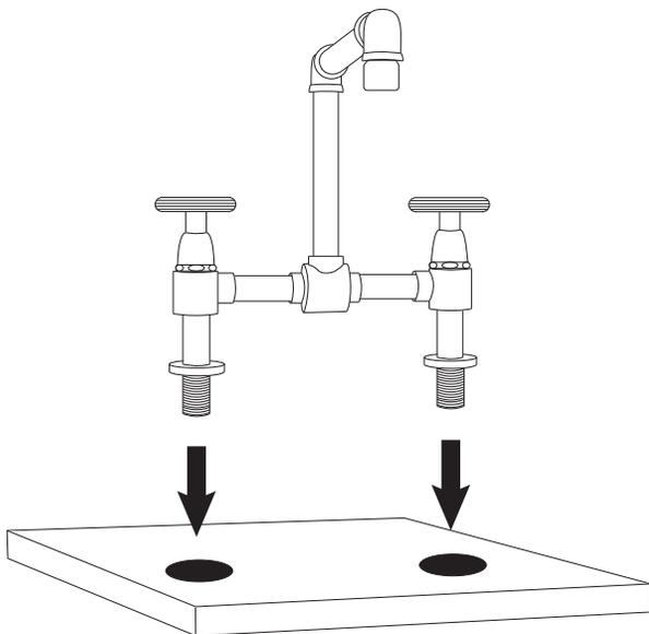
3. From beneath the sink, slide the rubber washers onto the faucet body. Thread the locknuts onto the threaded shanks until hand tight. Finish tightening using a basin wrench.
