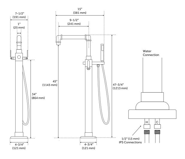
$\label{thm:condition} Underfloor\ access is\ required\ for\ proper\ installation.$  Installation on a concrete slab will require cutting and concrete removal.
