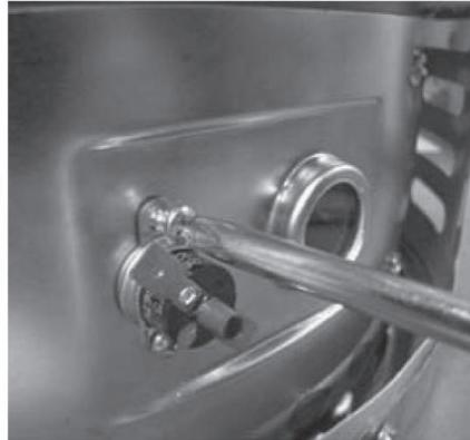
Step 5. Put new resettable thermal switch in place. Be sure contact surface of resettable thermal switch and inner door are free of any debris. Secure resettable thermal switch into place using screws from Step 4. **DO NOT OVER TIGHTEN SCREWS.**
