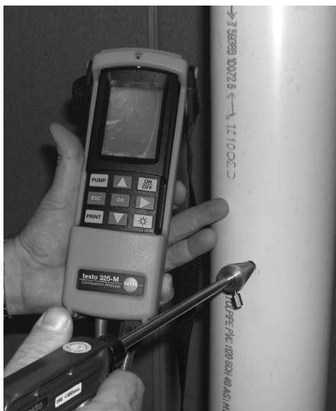
Figure 9.2: Insert Analyzer Test Probe into Test Port
