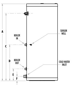
The "Hot Water Outlet" connection is Female NPT.
