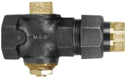
These valves are designed for use with natural, manufactured or LP gas only. All A.Y. McDonald 175 PSIG Gas Valves may be re-lubricated in the full open or the full closed position when the valve is pressurized or un-pressurized. All A.Y. McDonald plug style gas valves have factory set turning torque.
