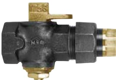
These valves are designed for use with natural, manufactured or LP gas only. All A.Y. McDonald 175 PSIG Gas Valves may be re-lubricated in the full open or the full closed position when the valve is pressurized or un-pressurized. All A.Y. McDonald plug style gas valves have factory set turning torque.
