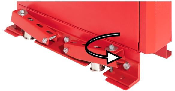
**Figure 2** Base Wheel Retraction
