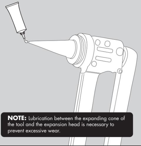
**NOTE:** Lubrication between the expanding cone of the tool and the expansion head is necessary to prevent excessive wear.
