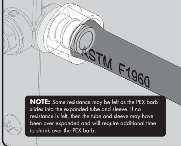
**NOTE:** Some resistance may be felt as the PEX barb slides into the expanded tube and sleeve. If no resistance is felt, then the tube and sleeve may have been over expanded and will require additional time to shrink over the PEX barb.
