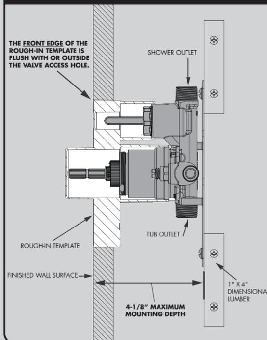
**5** Mounting Structure behind the wall must be capable of supporting the Valve in use. Following the rough-in dimensions for your model of valve (located at the end of this manual), reference the diagram below for the installation and placement of the bracing within a 2"x4" wall, using a 1"x4" brace. Mounting hardware is not included.
