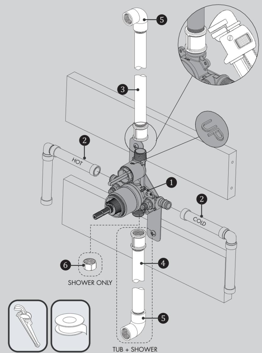
**NOTE:** The **HOT** water supply lines go into the H inlet, and the **COLD** water supply lines go into the C inlet. Do not use PEX or CPVC between the valve and spout.
