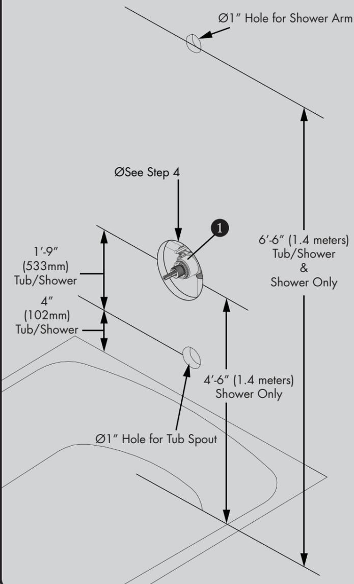
**4** Install the Rough-In Template over the Shower Valve being sure the Rough-In Template sits flush against Valve Body. Following the rough-in dimensions for your model of valve (located at the end of this manual) as well as the markings on the supplied Rough-In Template, install valve at proper depth. The distance from the Valve mounting surface to the finished wall **MUST** be between 3-1/8" - 4-1/8". See images below for reference.
