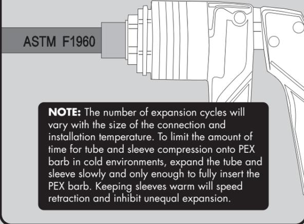
**NOTE:** The number of expansion cycles will vary with the size of the connection and installation temperature. To limit the amount of time for tube and sleeve compression onto PEX barb in cold environments, expand the tube and sleeve slowly and only enough to fully insert the PEX barb. Keeping sleeves warm will speed retraction and inhibit unequal expansion.
