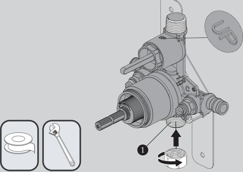
**7** Referencing the Rough-In Drawing, mount the Valve Assembly **1** to structure within the wall. Ensuring the Shower Outlet **2** and Tub Outlet **3** are positioned perfectly vertical. Mounting Hardware and Mounting Structure must be capable of supporting the Valve in use. Mounting hardware is not included.
