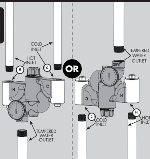
**WARNING:** The Valve will not function in the way it is intended to if Cold water supply pipe is connected to "H" Inlet on Valve and Hot water supply pipe is connected to "C" inlet on Valve.
