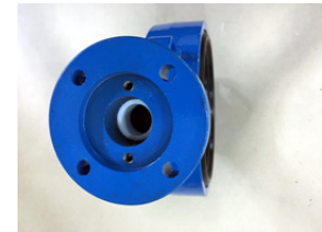
6. Insert bushing(s) into the upper stem hole. Note that 14" and larger valves have a long bushing that should be installed first.
