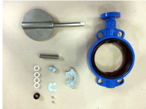
1. Insert the seat into the body, making sure the holes in the seat align with the stem holes in the body. Improper alignment can cause seat tears when stems are inserted.
