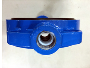
2. Insert bushing(s) into the lower stem hole. Check the valve's bill of materials for correct quality and type of bushings.
