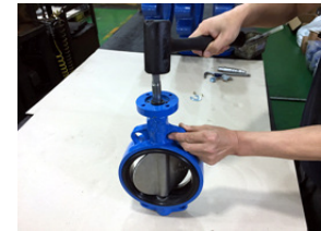
9. If necessary, drive the upper stem into the disc with a rubber mallet. If there is much resistance, make sure the stem flats are aligned appropriately to the disc.
