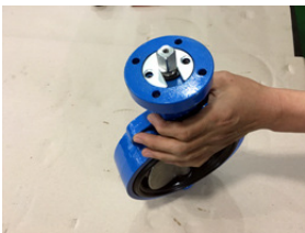
10. Slide the retaining plate onto the groove located just below the square drive of the stem. Align the screw holes with the holes in the body's top flange.
