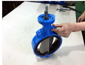
8. With lubricant, insert the upper stem almost all the way into the body. Make sure the stem flats are aligned with the receiving hole in the disc.
