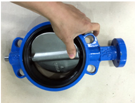
4. Insert the bottom of the disc into the seat over the lower stem. With the disc in the partially open position, push or tap the top of the disc to align with the upper stem hole.
