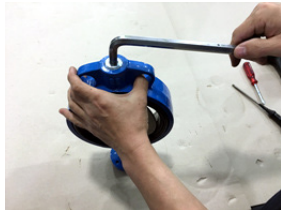
13. Screw the lower stem plug in place using a hex wrench. Do not overtighten the plug on lower stem.
