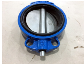
5. Insert the lower stem into the disc by pushing the valve body and disc assembly down onto the stem. Then tap the lower stem further in beneath the internal threads in the body.
