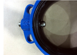
3. With lubricant, insert the lower stem into the body. Push the stem so that just the tip comes through the seat.
