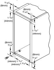
Fig. 28 – Leveling Legs Location Relative to Cooling Equipment
