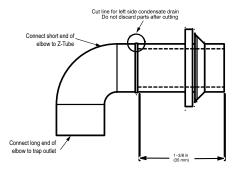
Fig. 16 – Modify Rubber Drain Elbow
