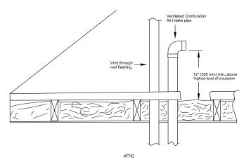
Fig. 49 – Vent Terminations for Ventilated Combustion Air<sup>A10497</sup>
