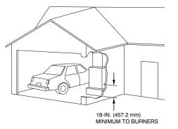
Fig. 5 – Installation in a Garage
