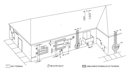
Fig. 43 – Ventilated Combustion Air and Non-Direct Vent Termination Clearance
