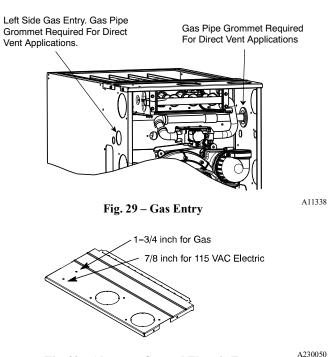
Fig. 30 – Alternate Gas and Electric Entry
