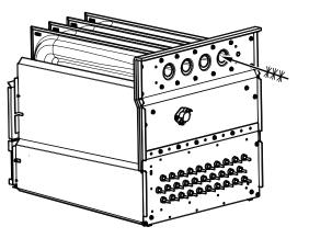
Fig. 70 – Cleaning Heat Exchanger Cell
