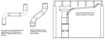
Fig. 56 - Near Furnace Vent Connections
