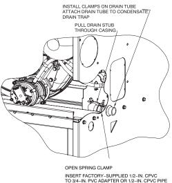
TO 3/4-IN. PVC ADAPTER OR 1/2-IN. CPVC PIPE \*CLAMP MAY BE LOCATED ON OUTSIDE OF DRAIN
