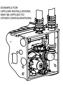
Fig. 45 – Sample Inlet Air Pipe Connection for Polypropylene<sup>A12220</sup> Venting Systems
