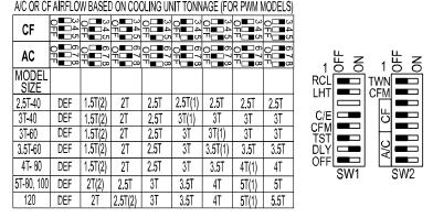
1. Default A/C airflow when A/C setup switches are in OFF position.
