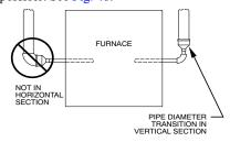
Fig. 48 – Combustion Air and Vent Pipe Diameter Transition<sup>A93034</sup> Location and Elbow Configuration
