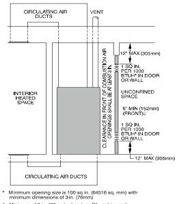
† Minimum of 3-in. (76mm) when type-B1 vent is used.
