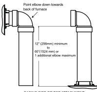
CASING SIDE OR TOP ATTACHMENT COMBUSTION AIR PIPE (NON-DIRECT VENT FOR ALL MODELS EXCEPT MODULATING UNLESS INSTALLED IN ATTIC OR CRAWL SPACE)
