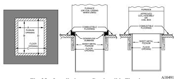
Fig. 25 – Installation on Combustible Flooring
