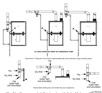
Fig. 51 – Recommended Combustion Air Inlet Moisture Trap
