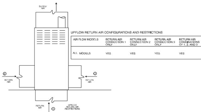
**Fig. 18 – Upflow Return Air Configurations and Restrictions** A190270
