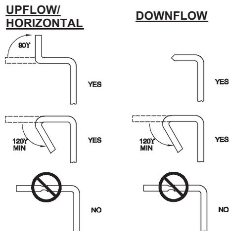
**Fig. 16 – Duct Flanges**
