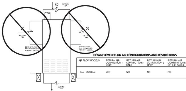
**Fig. 17 – Downflow Return Air Configurations and Restriction** A190271
