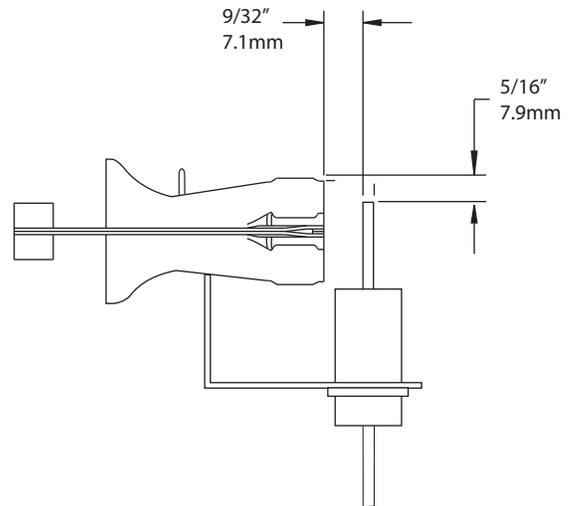
Fig. 50 – Igniter Position - Side View
