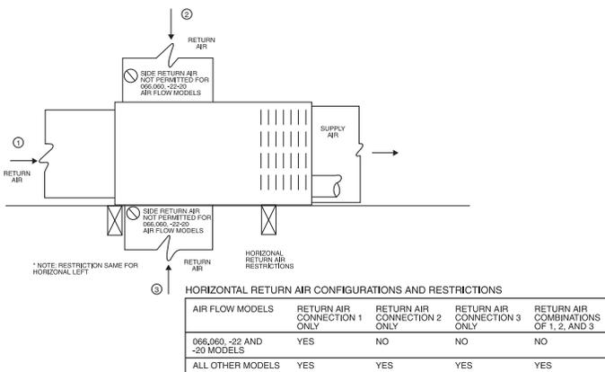
**Fig. 19 – Horizontal Return Air Configurations and Restrictions** A02162
