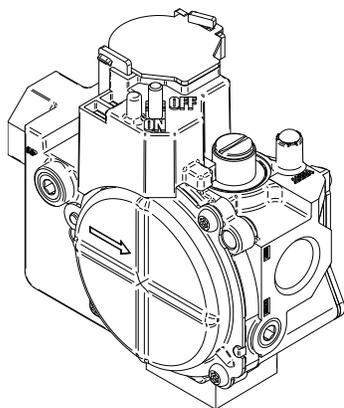
**Fig. 20 – Redundant Automatic Gas Control Valve**
