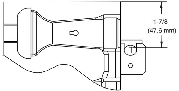
Fig. 49 – Igniter Position - Top View
