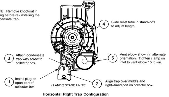
**Fig. 10 – Horizontal Right Trap Configuration**
