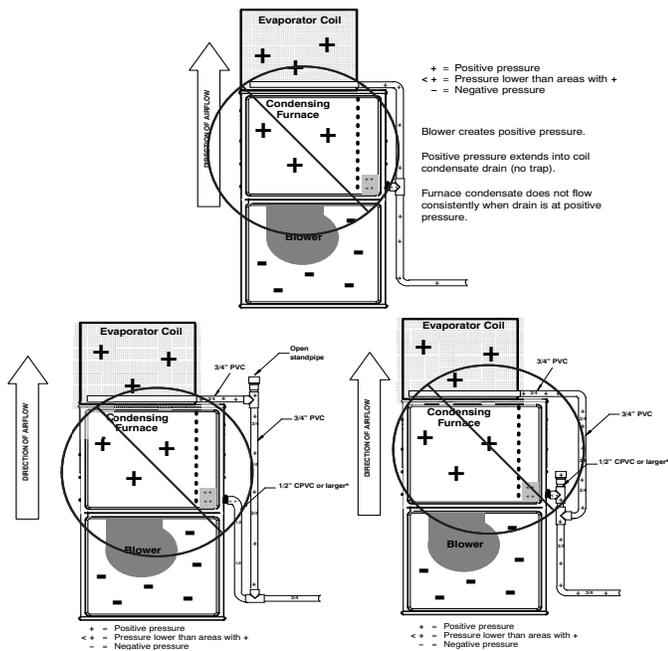
**Fig. 13 – Example of Field Drain Attachment (Not Allowed)**
