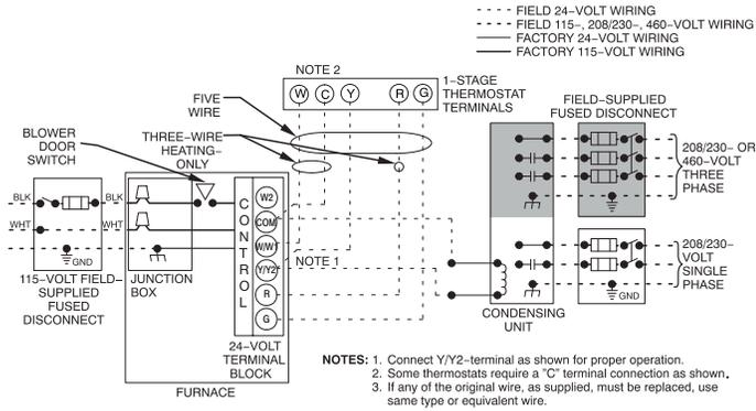
Fig. 32 – Typical Two-Stage Field Wiring Diagram
