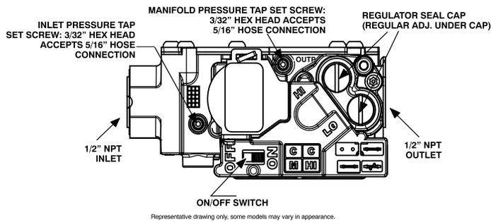
**Fig. 63 – Gas Valve with Tower Pressure Ports**
