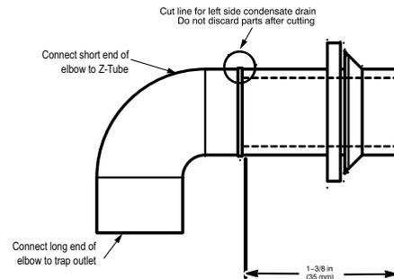
**Fig. 16 – Modify Rubber Drain Elbow**
