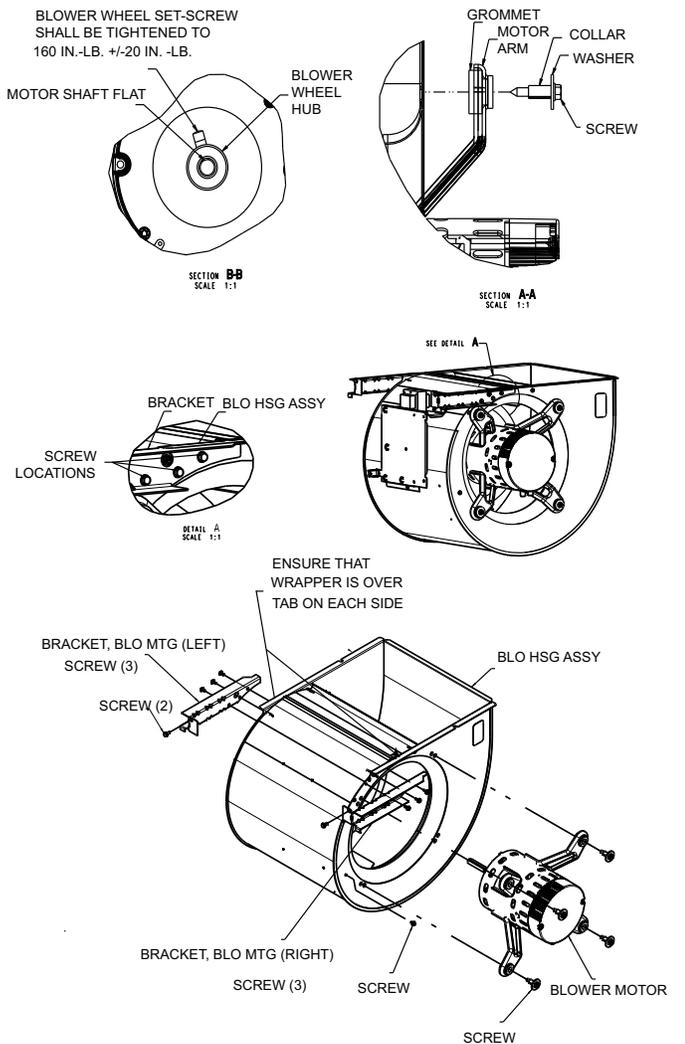
**Fig. 66 – Blower Assembly on 100V21--221002122**
