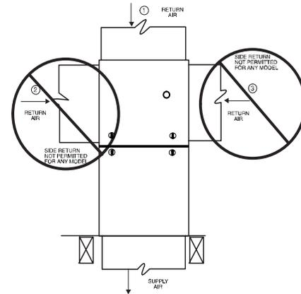
**Fig. 22 – Downflow Return Air Configurations and Restrictions**
