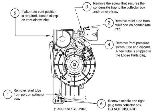
**Unconverted Factory Trap Configuration**
