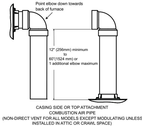
**Fig. 46 – Combustion Air Pipe Attachment** A13406
