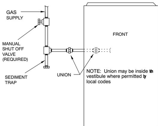
**Fig. 31 – Typical Gas Pipe Arrangement** A11035
