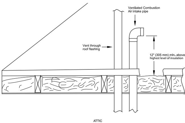
**Fig. 49 – Vent Terminations for Ventilated Combustion Air** A10497
