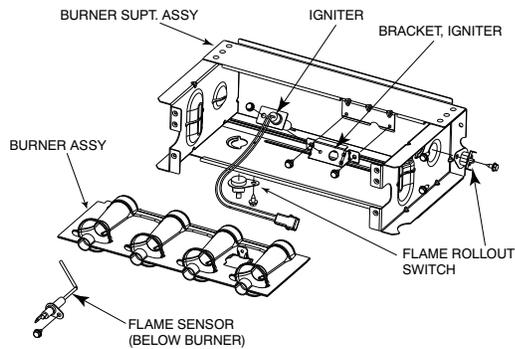
**Fig. 67 – Burner Assembly**
