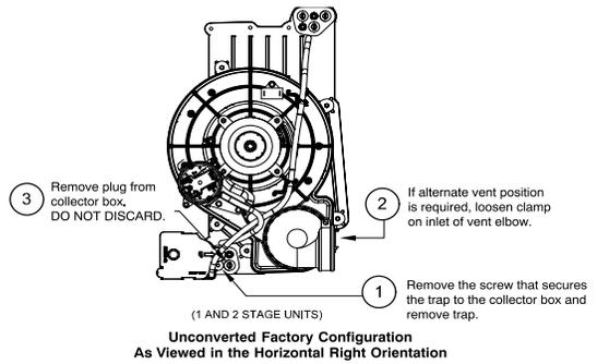
NOTE: Remove knockout in casing before re-installing the condensate trap.
