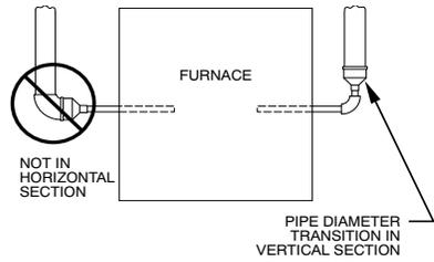
**Fig. 48 – Combustion Air and Vent Pipe Diameter Transition** A93034
