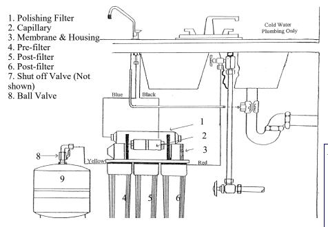
Reverse Osmosis is the process in which tap water is forced through a semi permeable membrane, leaving unwanted substance behind. These substances are rinsed away, resulting in fresh and clean drinking water. The WTRO-III is a five stage drinking water processor utilizing fibrous sediment filters, high grade Carbon Block filters, a Thin Film Composite R.O. Membrane and Metal Storage tank.
