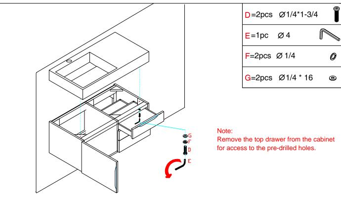
Step 7: Attach washbasin to the top of cabinet, insert the bolt through the Spring Washer (F) and the Flat Washer (G) through the underneath of corner block by Allen wrench.
