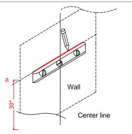
Step 2: Draw a horizontal line from the point a by using a leveler. (suggested H30" from floor to "a" line)
