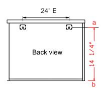
Step 1: Metal plates has been pre-installed to the back of cabinet, measure the distance between the bottom of the cabinet and point a.
