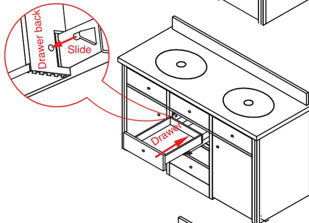
3. Align drawer back board hole and slide the hook of slide end, push the hook will slide into the hole.
