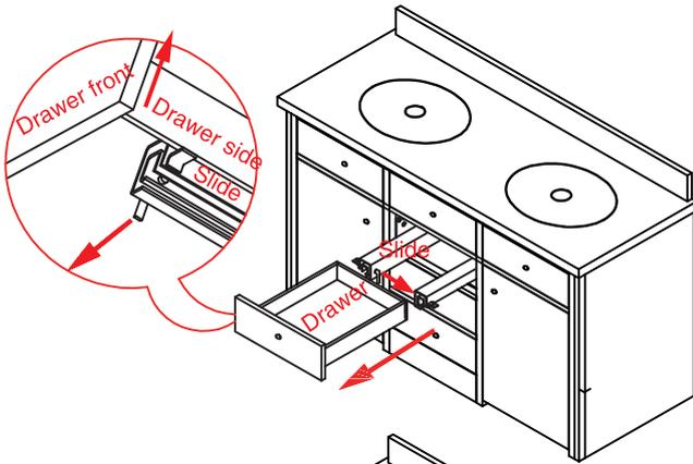
1. For removal, pull out the locking pin from the drawer side. Lift the drawer and pull it out from the cabinet.
