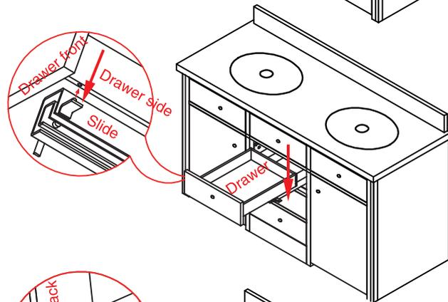
2. For the assembly of drawer, pull out the drawer member of the slide from the cabinet, lay the drawer onto the slide.
