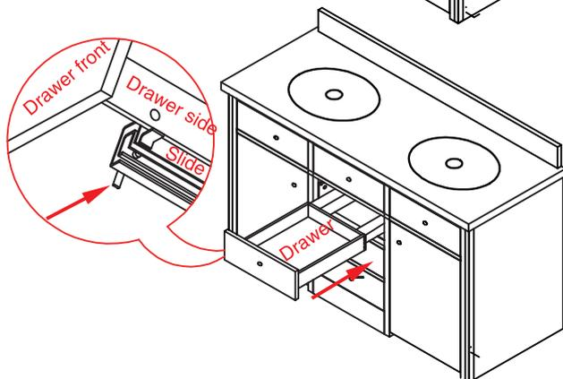
4. Press the locking pin into the drawer side hole to lock the position of the drawer.
