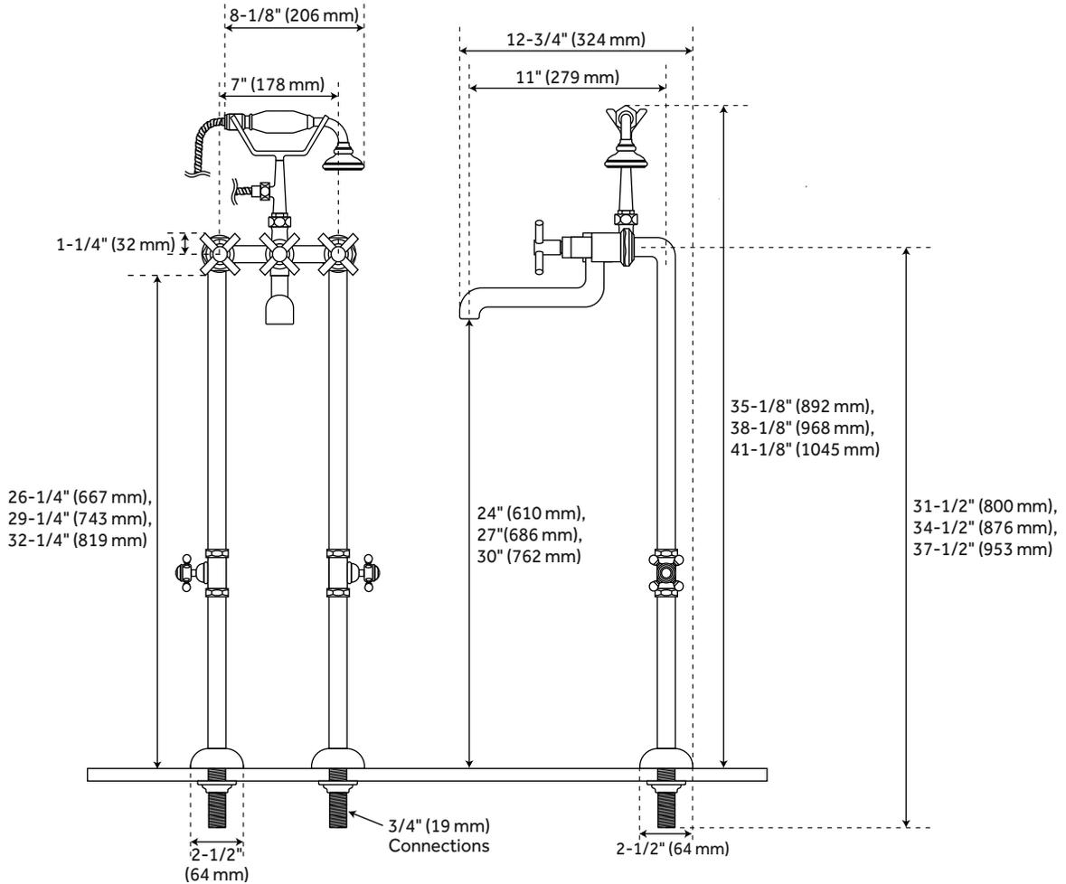
Underfloor access is required for proper installation.
