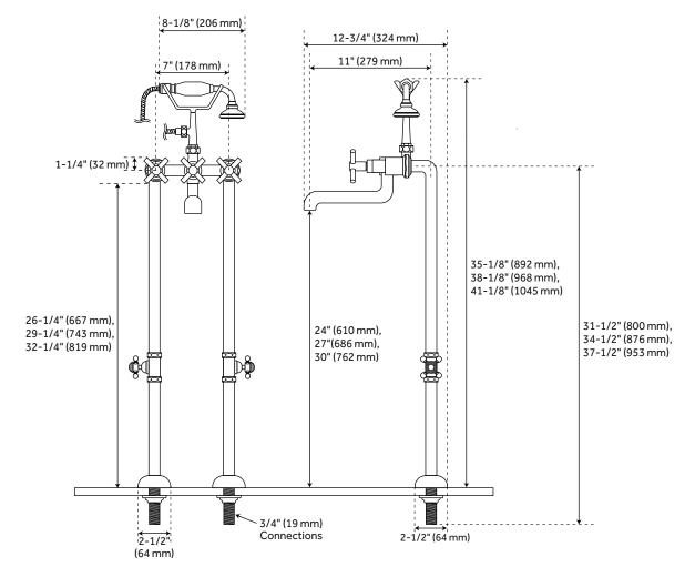
Underfloor access is required for proper installation. Installation on a concrete slab will require cutting and concrete removal.
