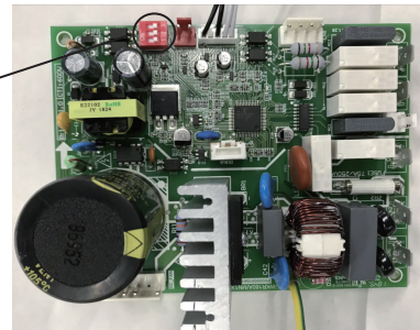
The location of SW3 Switch in the PCB Board
