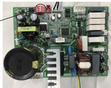
The location of SW3 Switch in the PCB Board
