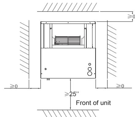
Fig.3 CLEARANCES IN THE VERTICAL POSITION
