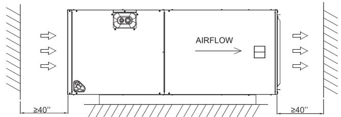
Fig.2 CLEARANCES IN THE HORIZONTAL POSITION
