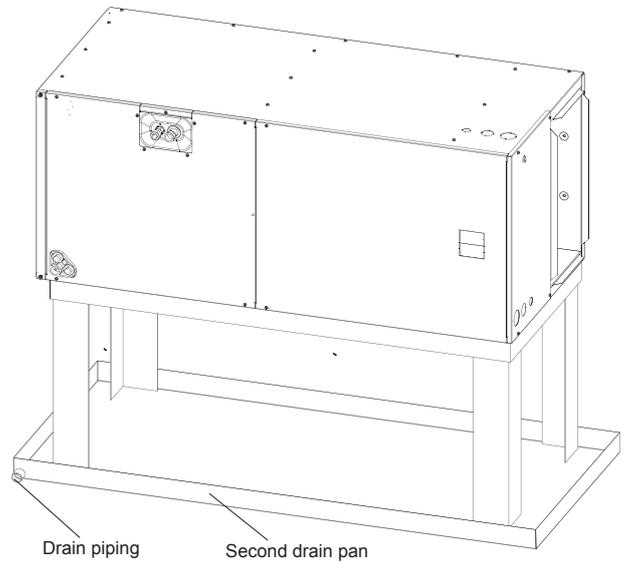
Fig.5 INSTALLED HORIZONTALLY
