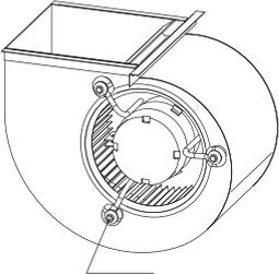
Make sure the blower motor support is tight (3-motor mount bolts) then check to see if wheel is secured to motor shaft before operating unit.
