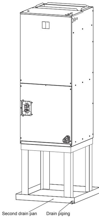
Fig.4 INSTALLED VERTICALLY
