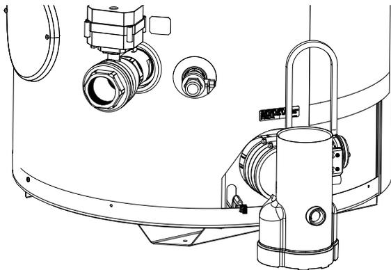
Figure 2 - Condensate Trap
