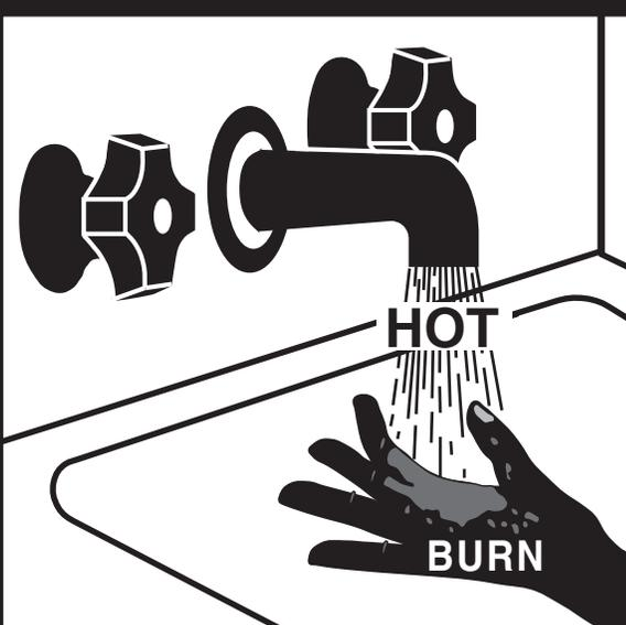
**Water temperature over 125°F can cause severe burns instantly or death from scalds.**
