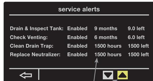
By selecting an option and then using the up and down arrow, you can set how often you’d like to be alerted to system maintenance.
