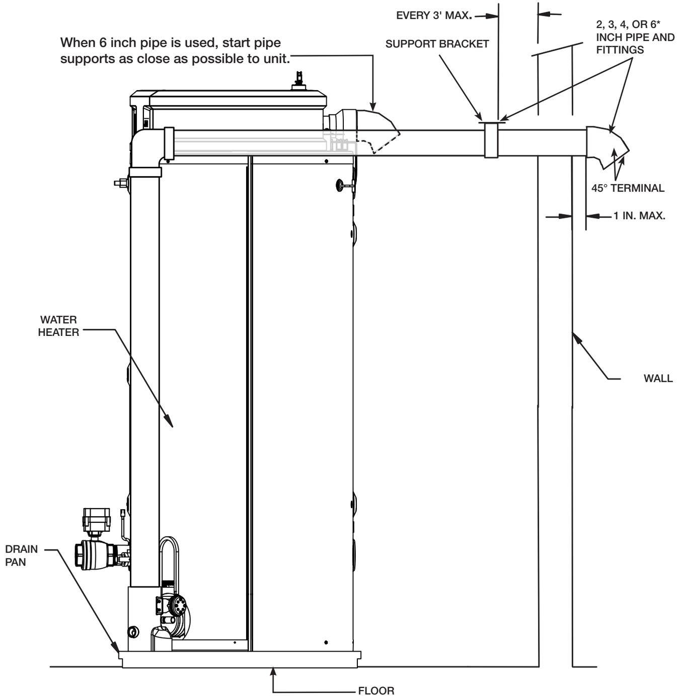
\* A 6 inch pipe can be used on 300,000 Btu/h models and above.
