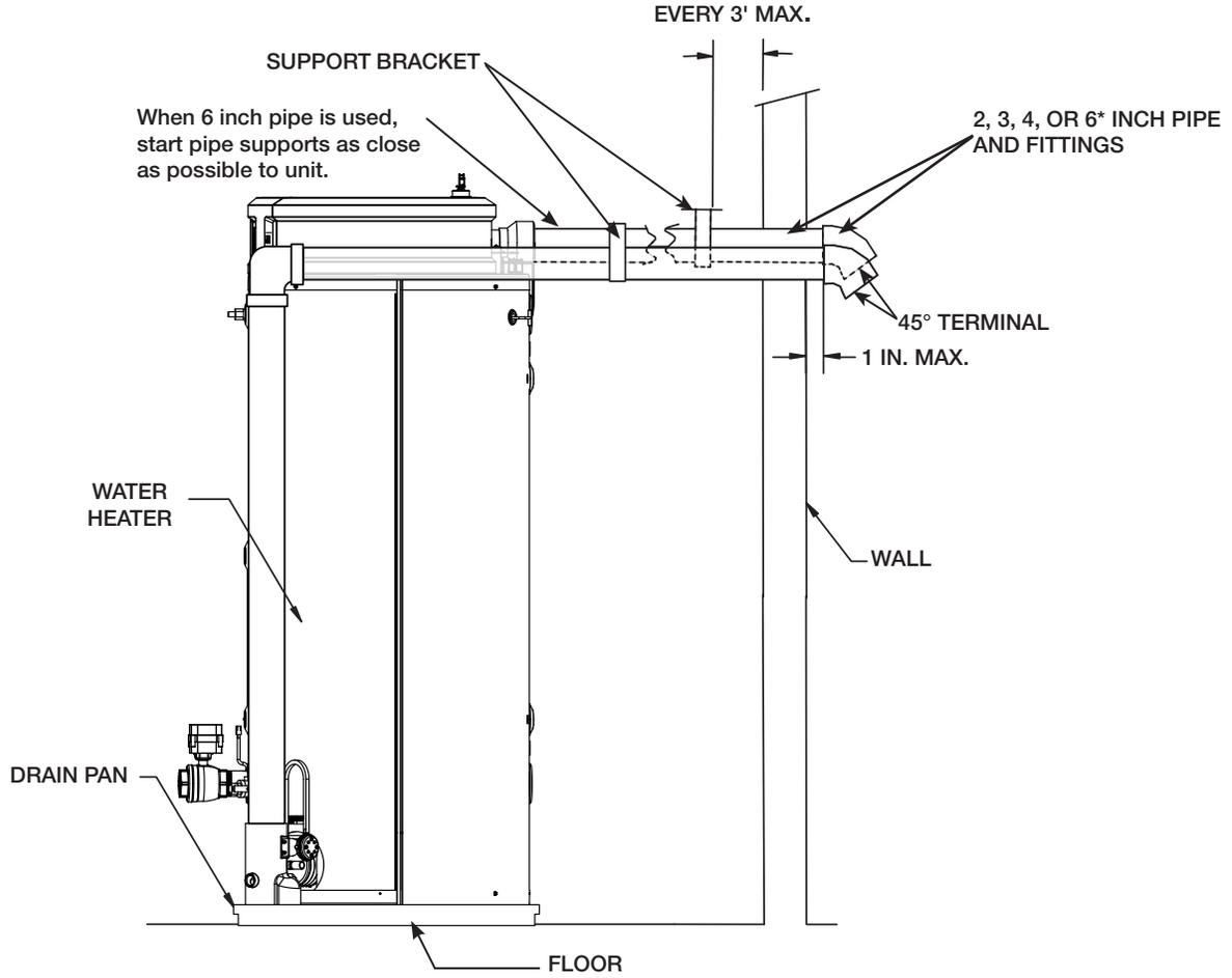
\* A 6 inch pipe can be used on 300,000 Btu/h models and above.
