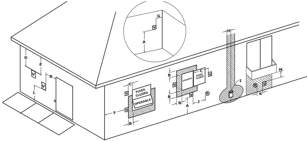
☑ VENT TERMINAL    ⊗ AIR SUPPLY INLET    ▨ AREA WHERE TERMINAL IS NOT PERMITTED
