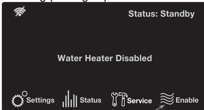
Press the enable button to turn the water heater on
