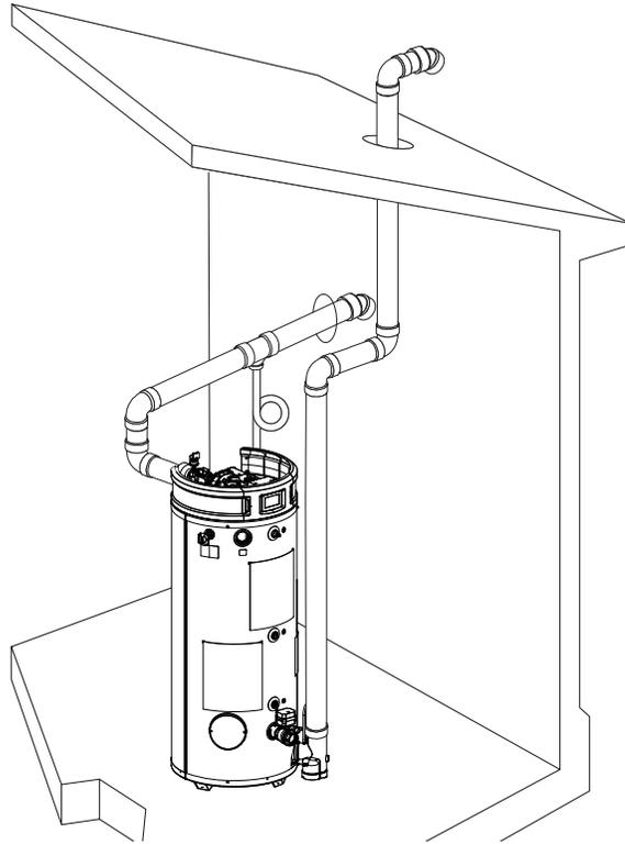
Direct Vent Horizontal Vent Vertical Intake
