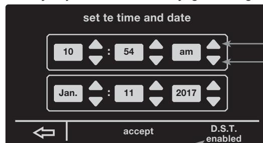
The D.S.T function allows you to adjust the time for daylight savings time.
