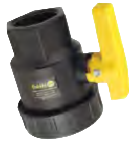
UNION BALL VALVES (BVMF) POLYPROPYLENE BODY EPDM O'RINGS TEFLON SEATS 100 PSI @ 72°F FPT THREADS
