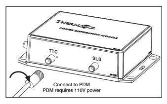
Connect the data cable to Power Distribution Module (PDM). (The other end of the cable runs to the back of the control in the shower location.)
