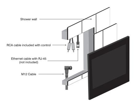
Route the M12 cable through the finished wall to the back side of the control. (The other end of the cable runs to the PDM location.) NOTE: It is recommended to run the cable through electrical conduit. DO NOT STAPLE the cable!
