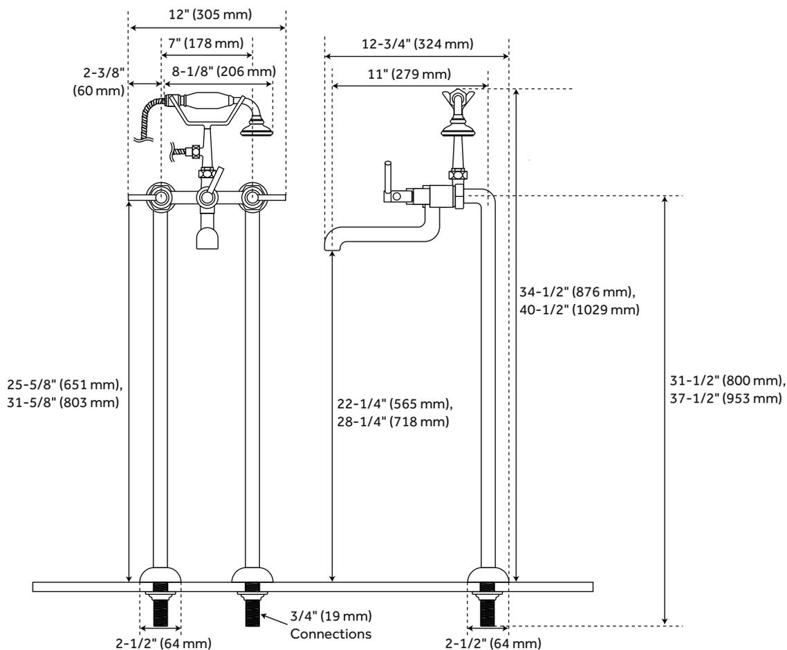
Underfloor access is required for proper installation.
