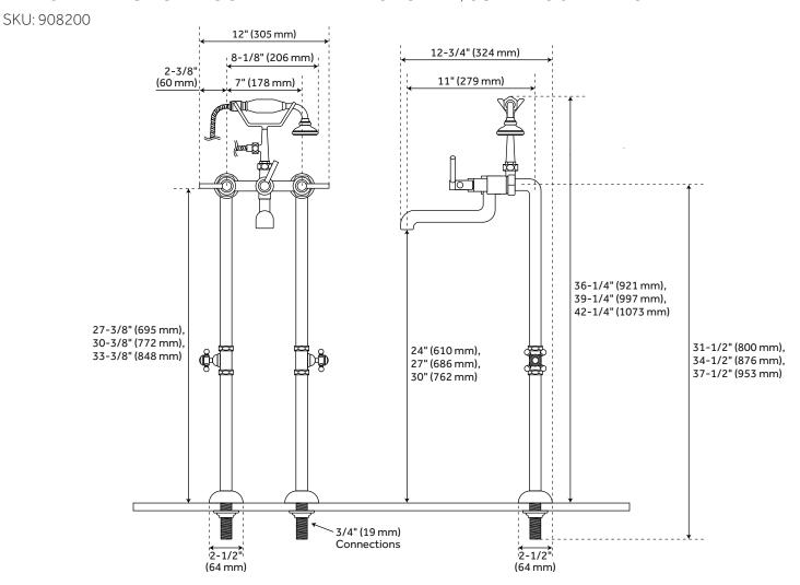
$\label{thm:condition} Underfloor\ access is\ required\ for\ proper\ installation.$  Installation on a concrete slab will require cutting and concrete removal.
