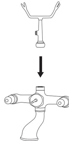
10. Attach the hand shower to the faucet by using the provided flexible hose. Connect the hose to the outlet located on the cradle. Place the hand-held shower in the cradle.
