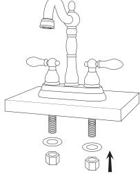
4. Connect the main water supply lines to the threaded shanks of the faucet. If necessary, use the provided brass nuts and cone washers to make the connections. Use an adjustable wrench to tighten, but be careful not to overtighten. Apply thread sealant or plumber's tape to the threads before attaching.
