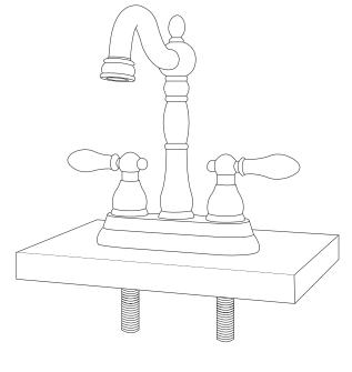
3. From below, slide each of the provided rubber washers onto the threaded shanks. Secure the faucet by tightening the provided lock nuts onto each shank. Hand tighten firmly.
