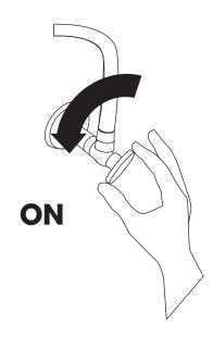
6. Remove the aerator from the faucet spout. Turn the faucet on to check for any leaks. Ensure that both hot and cold water are running properly. Allow the water to flow for approximately 60 seconds to remove any dust or loose sediment from the water lines. Reattach the aerator.
