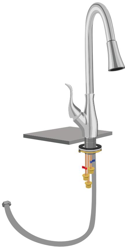
4. Attach the provided braided water lines to the copper supply tubes on the faucet. Apply plumber's tape or thread sealant to the threads before tightening. Ensure that you are connecting the hot and cold lines appropriately. Hand tighten the connections, then finish tightening with a ¼ turn using an adjustable wrench.
