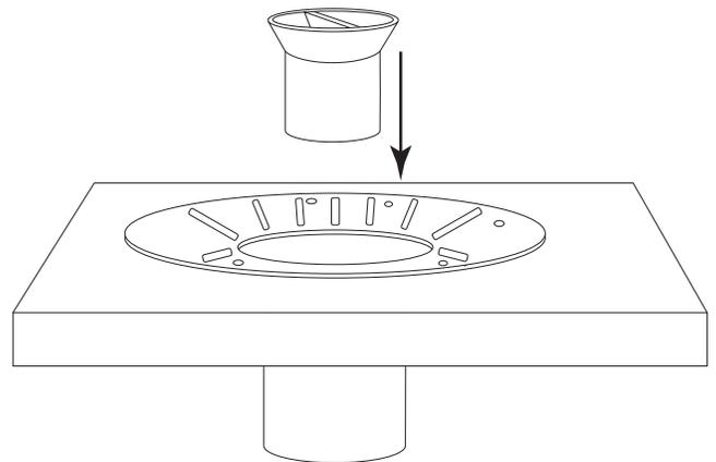
8. Turn the drain clockwise to lock into place, then secure the drain to the sub floor with screws.
