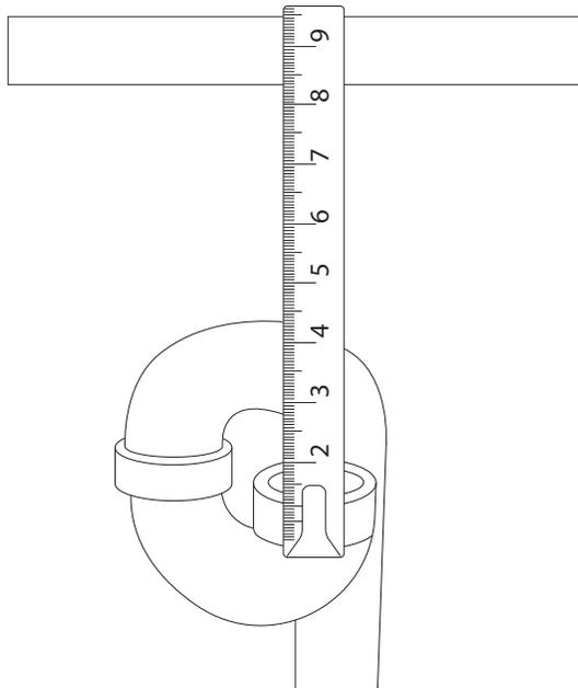
3. Cut the provided 1 1/2" PVC pipe 3" shorter than the distance between the floor and the p-trap (measurement taken in step two).
