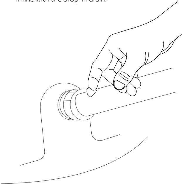
14. With caution, slowly drop the tub into position, inserting the tail piece into the drop-in drain.
