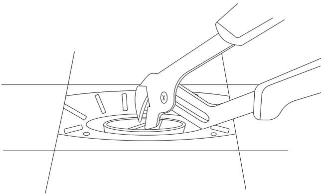
11. Once ready for tub installation, apply the provided lubricant to the rubber portion of the inside of the drain.
