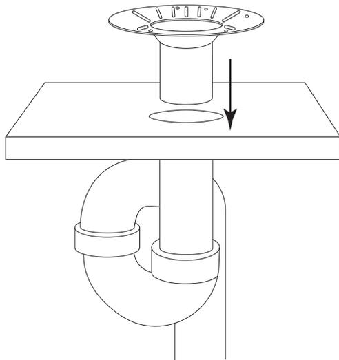
7. Insert the drain plug into the drop-in drain, if not already inserted.
