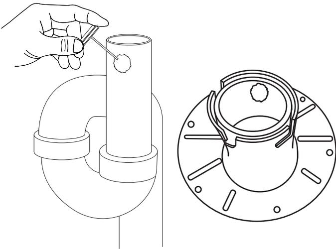
6. Slide the drop-in drain onto the PVC pipe, using a twisting motion to ensure proper cement bond, apply pressure until the cement is fully set. Ensure that the rim of the drop-in drain sits flush on the sub floor. Act quickly before cement sets.
