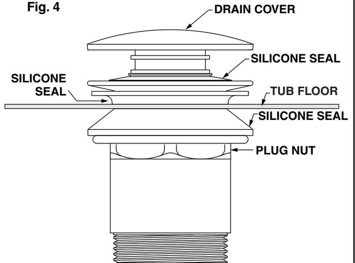
**4** Tighten drain nut using a pipe wrench and plug wrench. Make sure all of the silicone seals are in the proper location (as shown in Fig. 4) and there is no water leaking.
