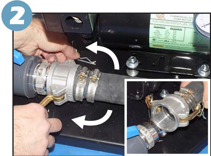
2 Loosen clamps on cam fitting & disconnect hose.
