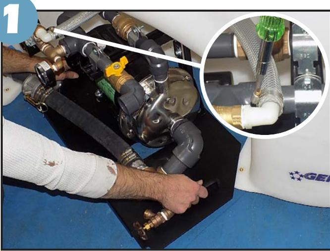
Using the handles on base, slide the left side of pump assembly into the tank opening & connect test hose.
