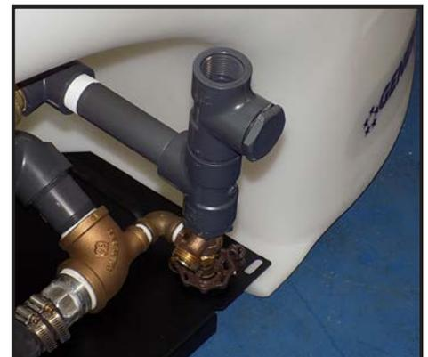
Thread the riser into manifold and tighten until riser is in an upright position.
