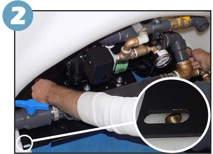
Position the pump assembly so the slots in the base line up with the nuts on both sides.
