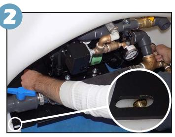
Position the pump assembly so the slots in the base line up with the nuts on both sides.
