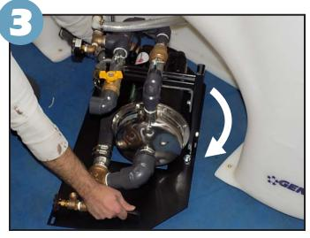
Slide the right side of pump assembly out first using the handles on the sides of the base plate.
