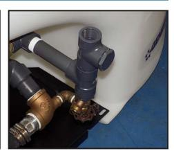
Thread the riser into manifold and tighten until riser is in an upright position.
