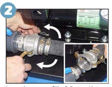
Loosen clamps on cam fitting & disconnect hose.
