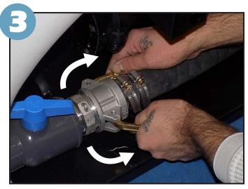
Install the hose & lock the clamps on cam fitting.
