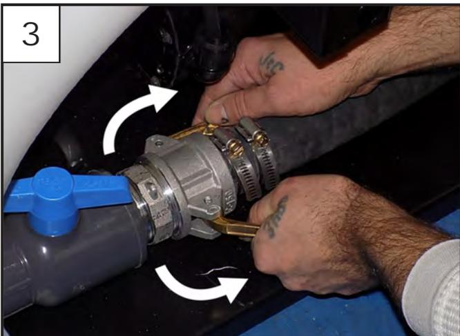
Install the hose & lock the clamps on cam fitting.
