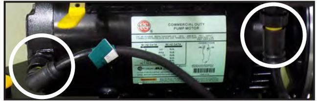
panel, the power cords to the pump and pressure switch will need to be disconnected / reconnected.
