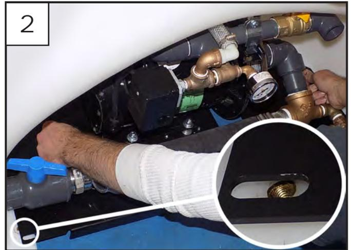
Position the pump assembly so the slots in the base line up with the nuts on both sides.
