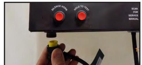
Connect alarm cord to socket and screw to tighten.
