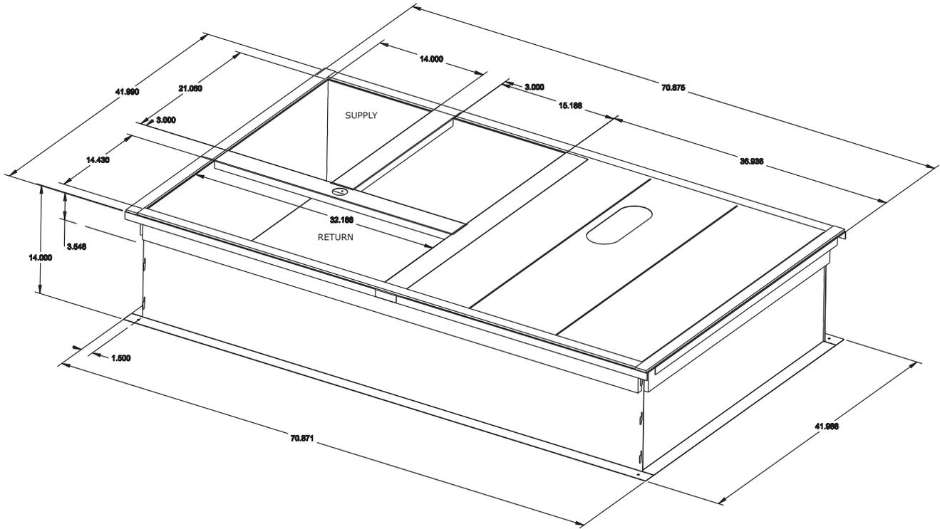
Figure 7. Downflow unit clearance — 3–5 tons standard efficiency
