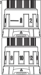
2. To use the driving mode rotate the torque selector collar until the desired clutch setting appears in line with the arrow.
