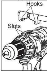
2. To remove the side handle, loosen the side handle grip until the side handle can be removed. Reposition and tighten securely.
