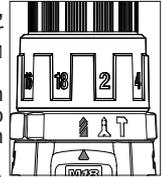
**NOTE:** The number selected on the torque selector collar has no effect on operation of the drill in drilling mode.
