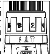
The adjustable clutch, when properly adjusted, will slip at a preset torque to prevent driving the screw too deep into different materials and to prevent damage to the screw or tool.
