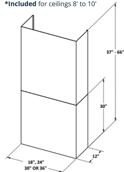
**DUCT COVERS:** MODEL #: PDC3230, PDC3236, PDC3242, PDC3248
