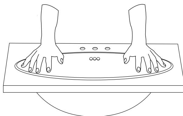
4. Apply a thin bead of silicone sealant around the perimeter of the sink, where the sink meets the countertop. This will prevent moisture from getting underneath the rim of the sink.
