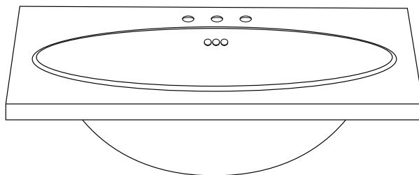
2. Remove the sink and run a bead of neutral cure silicone sealant around the underside of the rim.
